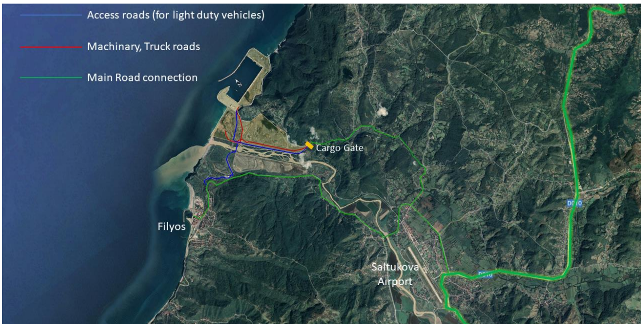
Figure 3-34: Access and Connection Roads – Construction
