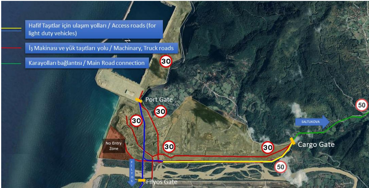
Figure 3-33: Access Roads - Construction
