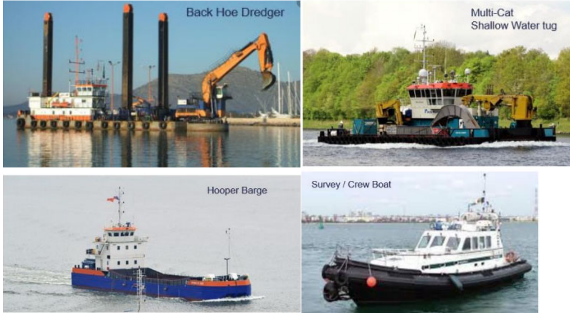
Figure 3-20: Typical Images of Vessels to Be Used at Near Shore Dredging
