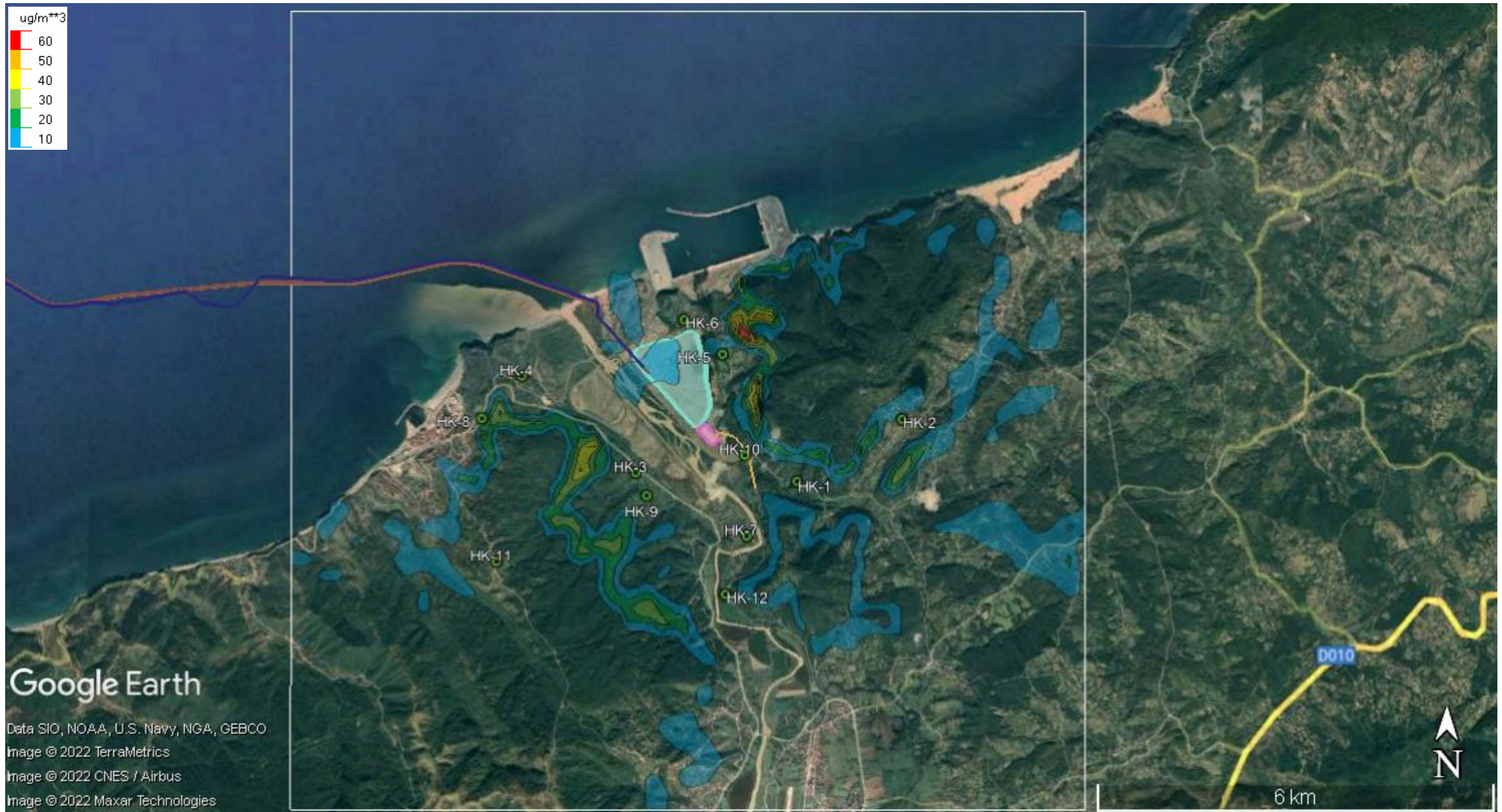
Figure 7-16: 1 st Highest 8-Hour Average GLCs for CO during Normal Operation ( \mu\text{g}/\text{m}^3 )
