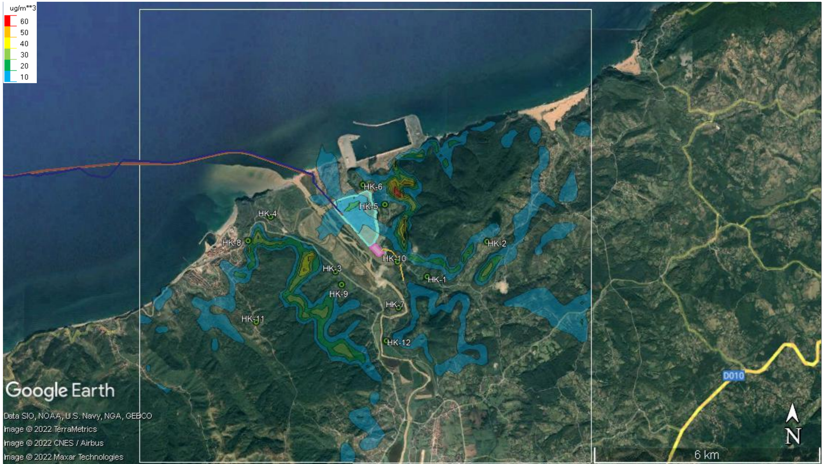
Figure 7-21: 8hr Average GLC for CO during Abnormal Operation ( \mu\text{g}/\text{m}^3 )
