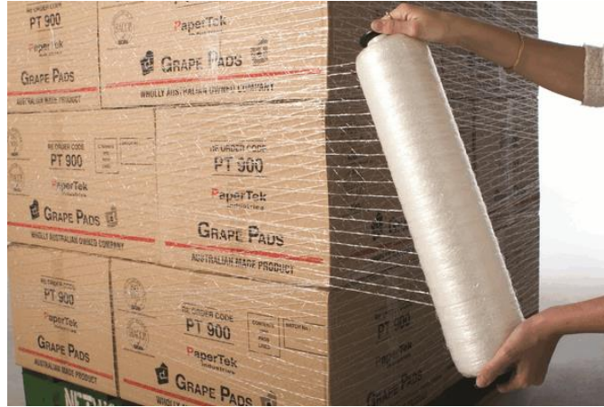
Figure 6 – Wrapping Film (Stretch Film) Technique
