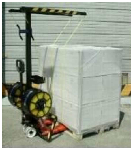
Figure 7 – Application of the Pallet Strapping
