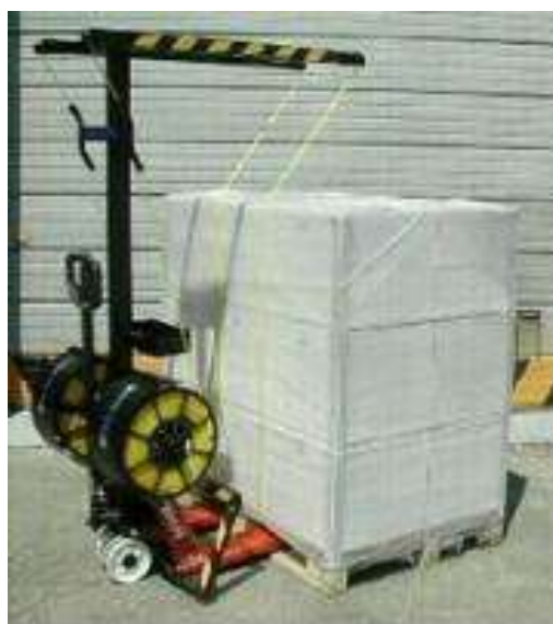
Figure 7 – Application of the Pallet Strapping
