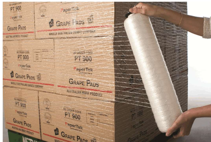
Figure 6 – Wrapping Film (Stretch Film) Technique
