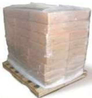
Figure 4 – Pallet covered with Polyethylene Shrink
